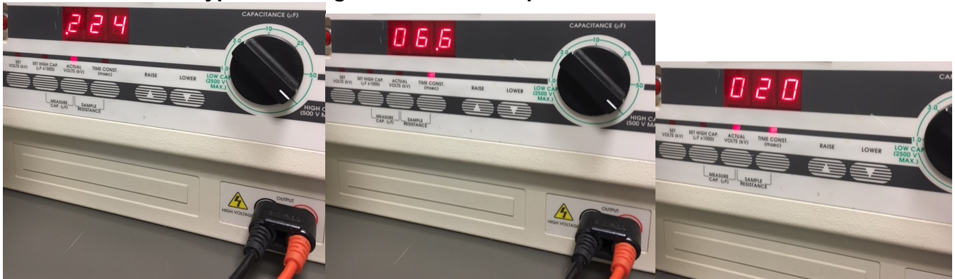
actual Volts: 224 V. Time constant: 6.6 ms. Sample resistance: 20 ohms
