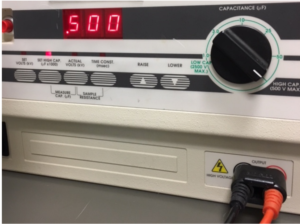
Set HIGH CAP ( \mu\text{F} \times 1000 ) to .500 (=500 \mu\text{F} )
